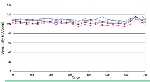
When sensors are tested monthly, their very good stability shows that they can be used in fixed sites, where maintenance and recalibration costs are important.
