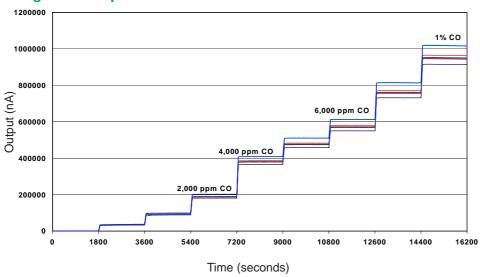
Figure 4 shows the response to step changes in CO concentrations from zero to 1% by volume.
