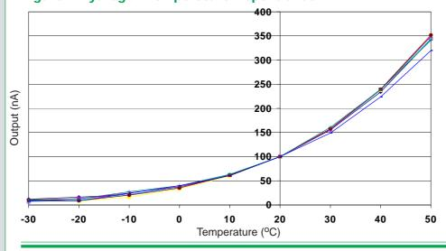
Hydrogen sensitivity is very dependent on temperature.
