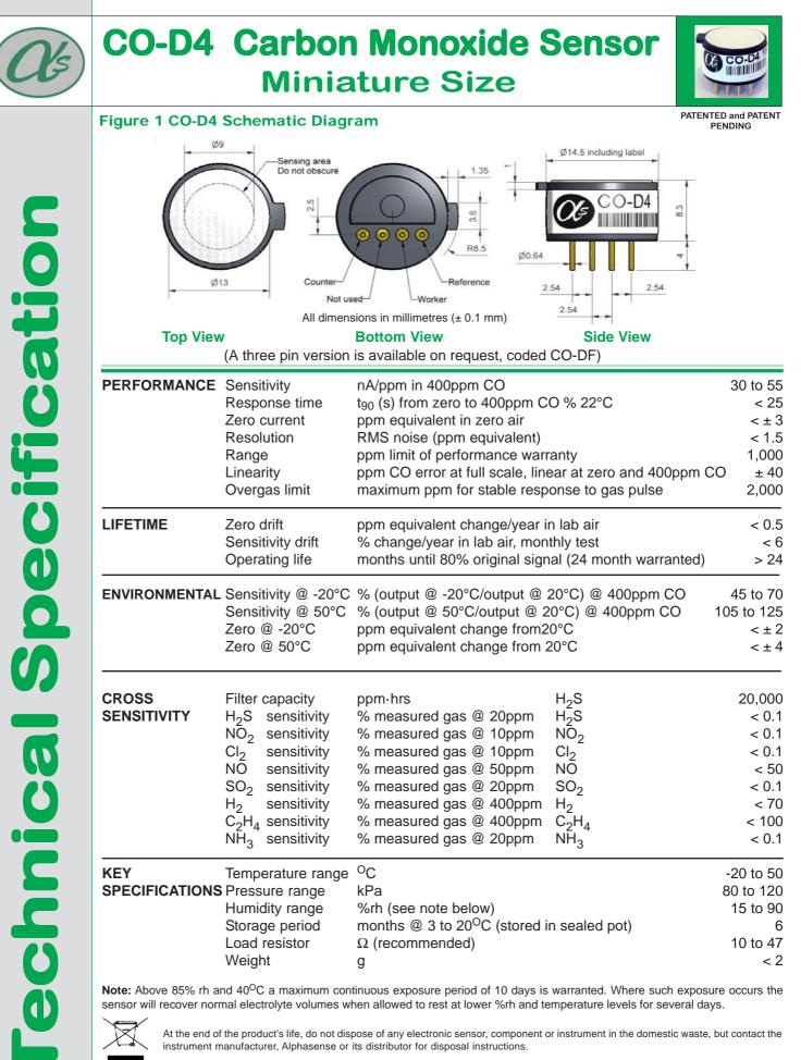
NOTE: all sensors are tested at ambient environmental conditions, with 10 ohm load resistor, unless otherwise stated. As applications of use are outside our control, the information provided is given without legal responsibility. Customers should test under their own conditions, to ensure that the sensors are suitable for their own requirements.
