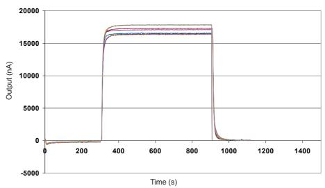
Figure 5 shows response to  $25ppm H_2S$ . Sensor shows a fast and stable response and recovery and repeatable sensitivity.
