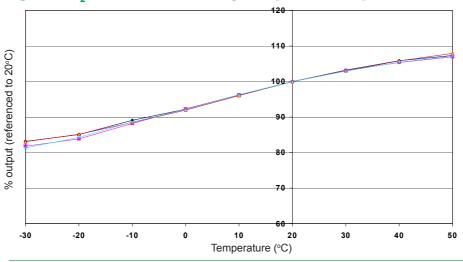
Figure 6 shows the % variation in sensitivity caused by changes in temperature.
