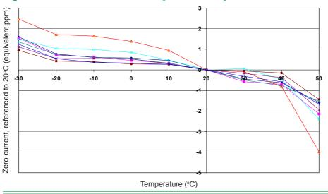
Figure 2 shows the variation in zero output caused by changes in temperature, expressed as ppm gas equivalent, referenced to the zero at 20°C.
