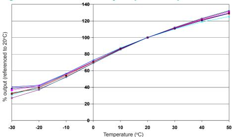
Figure 1 shows the % variation in sensitivity caused by changes in temperature.
