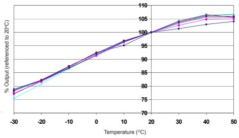
Figure 2 shows the temperature dependence of sensitivity at 2ppm H<sub>2</sub>S.
