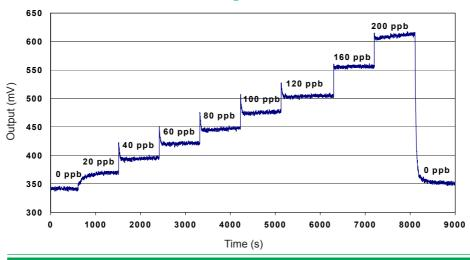
Figure 4 shows response to  $200ppb H_{\circ}S$ .
