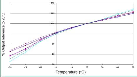
Figure 2 shows the variation of sensitivity at 25ppm HCI caused by changes in temperature.
