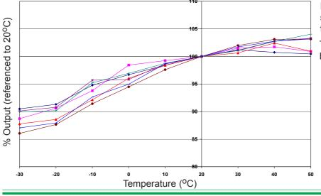
Figure 2 shows the variation in sensitivity caused by changes in temperature.
