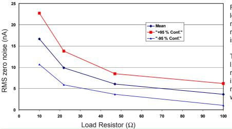
Figure 3 shows the effect of the load resistor on the RMS zero noise for the NO2-B1 sensor. The mean and  $\pm 95\%$  confidence intervals are shown.
