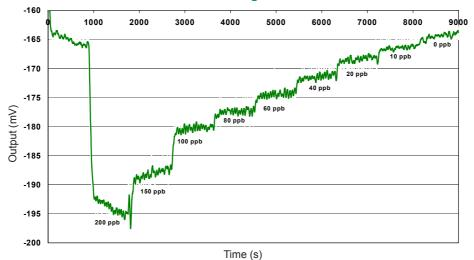
With a 33  $\Omega$  load resistor, the NO2-B42F shows excellent resolution, even at the ppb level: ideal for outdoor air environmental testing.
