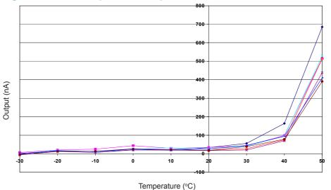
Figure 3 shows the variation in zero output of the working electrode caused by changes in temperature, expressed as nA.
