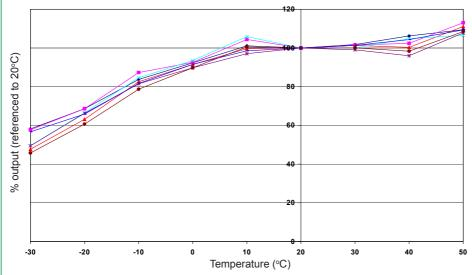
Figure 2 shows the temperature dependence of sensitivity at  $2ppm\ NO_2$ . This data is taken from a typical batch of sensors.
