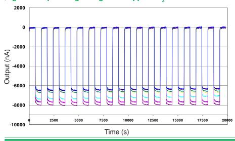
This hyteresis graph shows stable response when gassed repeatedly with 20ppm NO<sub>2</sub>
