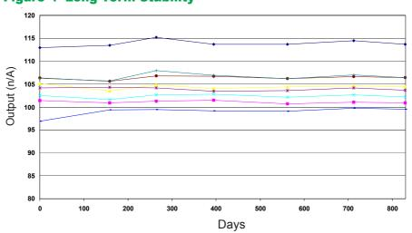
Mass flow Oxygen sensors show excellent long term stability. Regular calibration is not necessary so long as temperature compensation is correct.
