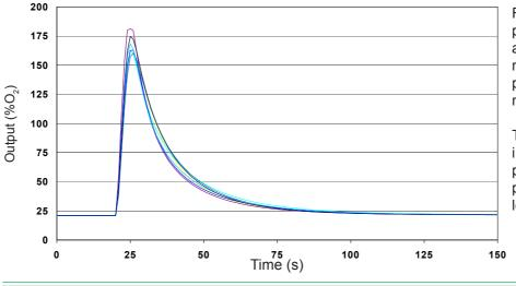
Figure 3 shows how a 25kPa pressure step change causes a signal transient that decays reproducibly. Negative pressure changes cause a negative transient.
