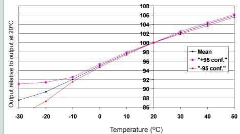
Figure 2 shows the variation of output caused by changes in temperature in 20.9% oxygen. The mean and  $\pm 95\%$  confidence intervals are shown.
