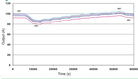
This time trace follows eight sensors' progress as they are first cooled to -30°C, then thermally stepped to +50°C before finally returning to 20°C.
