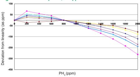
Sensor linearity is repeatable between sensors, allowing for software correction if required.
