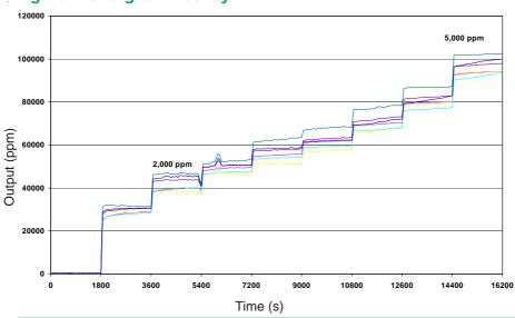
Sensors respond rapidly and are stable even at 5,000 ppm  $\text{PH}_{\text{q}}$ .
