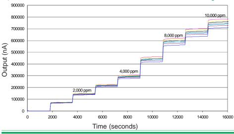
Figure 4 shows the response for a batch of sensors to high concentrations of SO<sub>2</sub> applied as sequential step increases.
