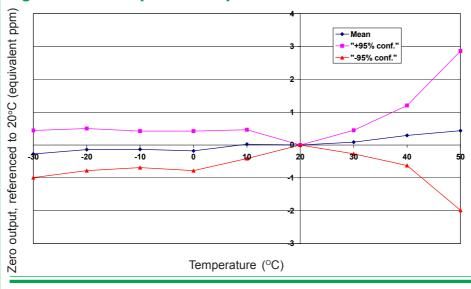
Figure 3 shows the variation in zero output caused by changes in temperature, expressed as ppm gas equivalent, referenced to zero at 20°C.
