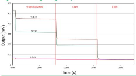
Figure 3 compares the output to 5 and 10ppm Isobutylene for 9.6 eV, 10.0 eV and 10.6 eV lamps.
