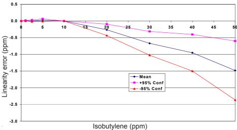
Reduced sensitivity at higher concentrations is a chemical/physical effect and can be corrected in software for a specific VOC.
