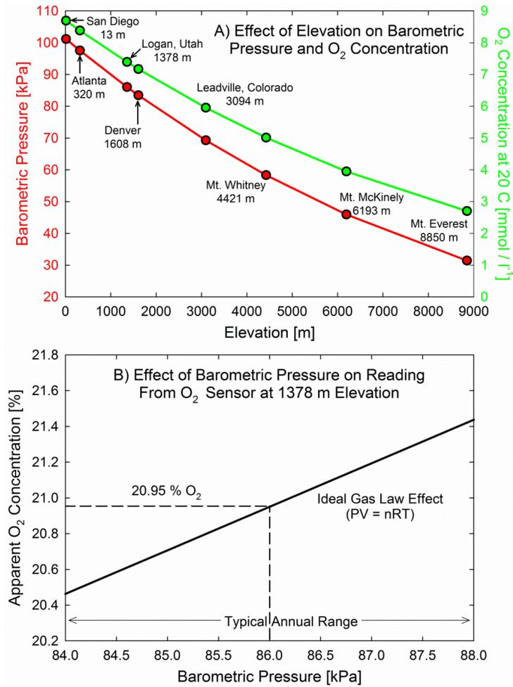
A) Barometric pressure and absolute oxygen concentration at 20 C as a function of elevation. Equation (6) was used to calculate barometric pressure.
