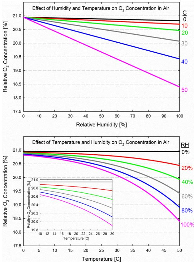
A) Relative humidity effects on relative oxygen concentration shown as a function of relative humidity at temperatures increments of 10 C and
