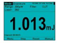
Exposure measurement (energy summing) with photodiode sensor.
