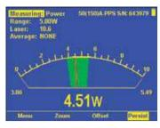
Analog needle display of power Persistence and min/max tracking.
