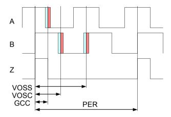
Figure 16: Calibration using incremental signals
