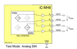
Figure 7: Output signals of the sine Hall sensors in test mode Analog SIN
