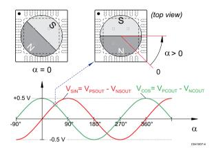
Figure 5: Pattern of the analog sensor signals with the angle of rotation
