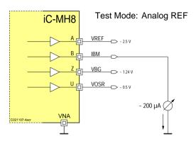
Figure 10: Setting bias current IBM in test mode Analog REF
