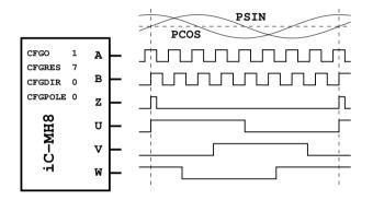
Figure 21: ABZ and UVW single ended signals
