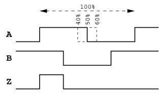
Figure 17: ABZ signals and relative accuracy
