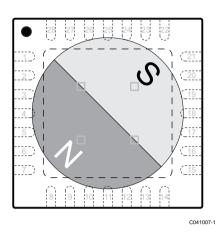
Figure 4: Zero position of the magnet
