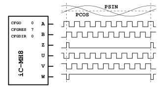
Figure 20: ABZ differential incremental signals
