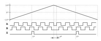
Figure 18: Quadrature signals for rotating direction reversal (hysteresis 1.4°)
