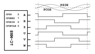
Figure 22: UVW differential commutation signals
