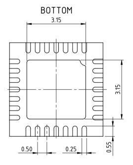
All dimensions given in mm. Tolerances of form and position according to JEDEC MO-220.
