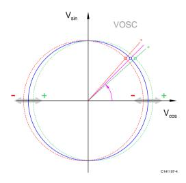
Figure 14: Effect of the cosine offset setting
