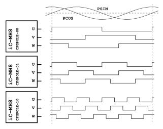
Figure 19: UVW signals for different settings of CFGPOLE
